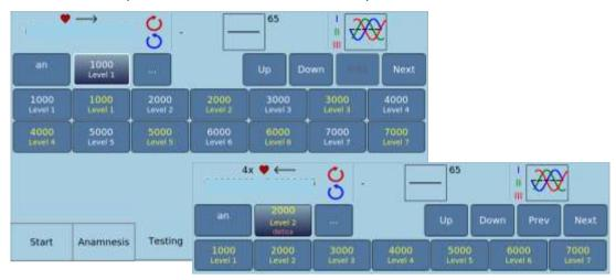
If a frequency program is called up, the "Cascade" key switches back and forth between the ascending and descending wobbled program.
